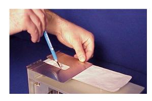
2. Determine location on the tray from where the sample will be cut. Place the tray flange under the hinged template and push down trapping the seal over plastic insert. Using the supplied trimming knife, cut out the sample sides. Make sure the blade used is sharp so that the lid is cut during the first attempt.
