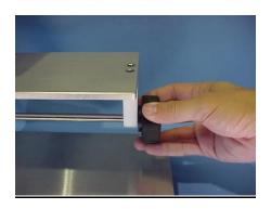
Adjust the tray support height on both the universal sample cutter and the HST 180T instrument to suit the tray to be tested.
