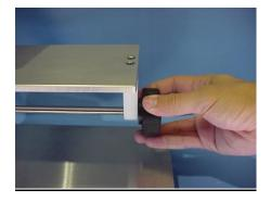
1. Adjust the tray support height on both the universal sample cutter and the HST 180 instrument to suit the tray to be tested.
