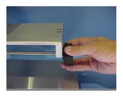
1. Adjust the tray support height on both the universal sample cutter and the HST 180 instrument to suit the tray to be tested.
