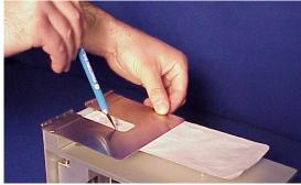
2. Determine location on the tray from where the sample will be cut. Place the tray flange under the hinged template and push down trapping the seal over plastic insert. Using the supplied trimming knife, cut out the sample sides. Make sure the blade used is sharp so that the lid is cut during the first attempt.
