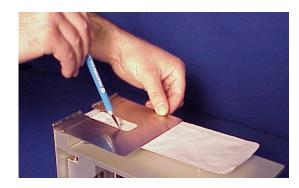
2. Determine location on the tray from where the sample will be cut. Place the tray flange under the hinged template and push down trapping the seal over plastic insert. Using the supplied trimming knife, cut out the sample sides. Make sure the blade used is sharp so that the lid is cut during the first attempt.
